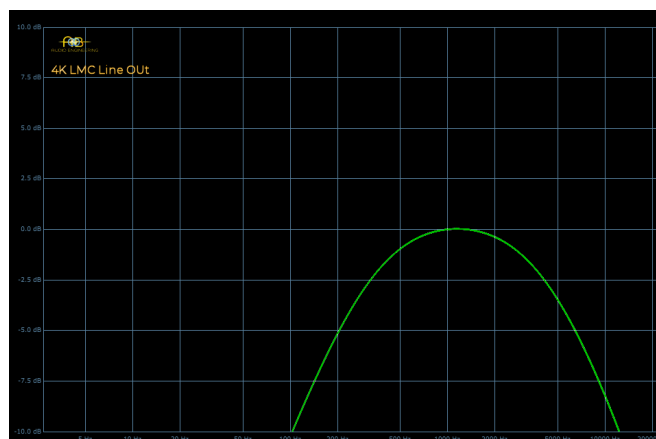
4K LMC Line Out frequency response (@ 0dBVU)
